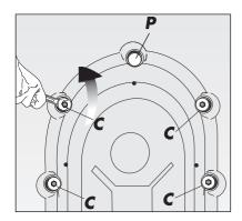
The transport safety bolts must be removed before any operation of the machine. Bolt heads, marked "C".
